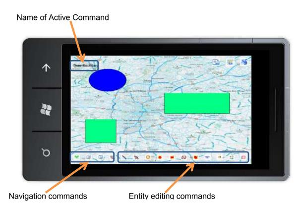
The figure above shows the toolbars for the 2 different types of the commands. The name of the active command is displayed on the top-left corner of the view.
